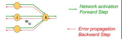
Backprop adjusts the weights of the NN in order to minimize the network total mean squared error.
